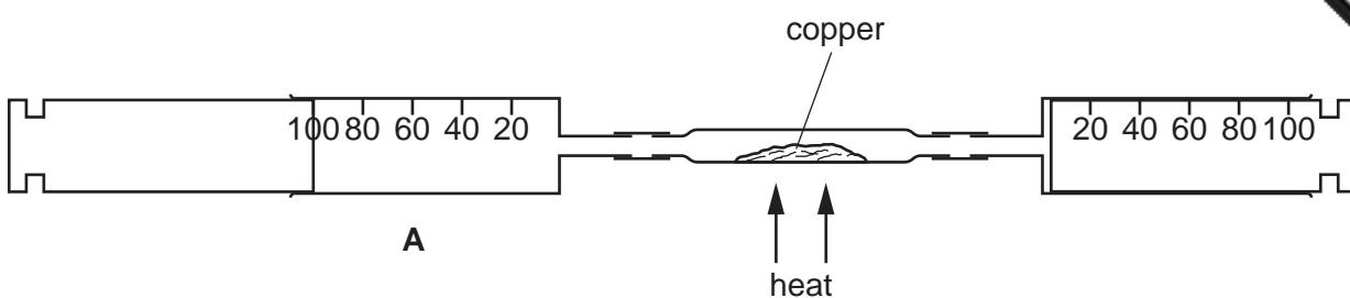
Syringe A contains 100 cm<sup>3</sup> of air. The air is forced backwards and forwards over the heated copper until the volume of gas forced back into the syringe A is constant.
